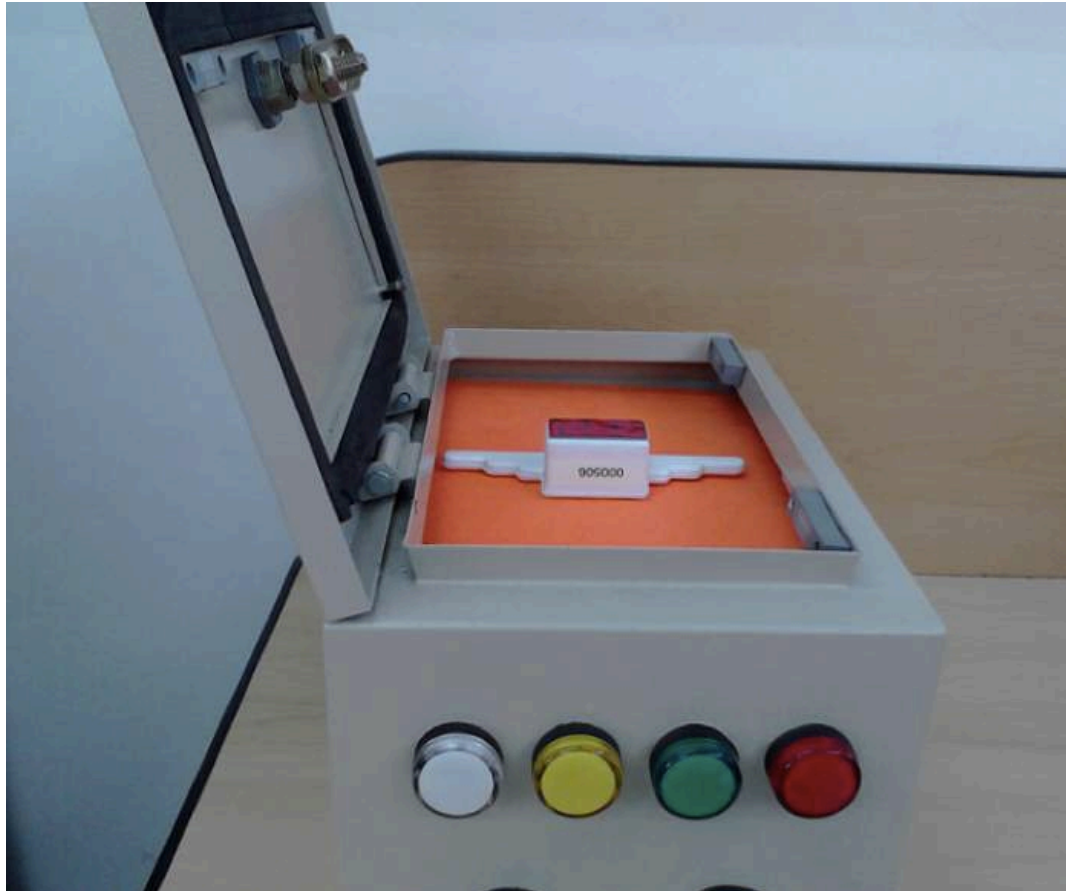
Tag Initialization Equipment for Field Operations and a Brasil-ID Reading/Writing Systems which is connected to the Central BackOffice for security and Access Keys management
